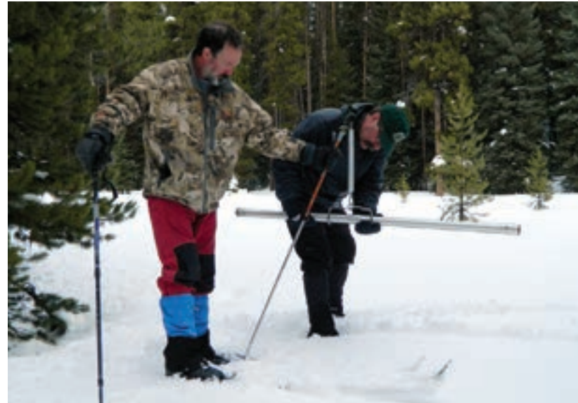
Left, icicles build up on Forest Service backcountry ranger Kraig Lang's mustache on a frigid snow sampling trip in the Bob Marshall Wilderness. Below, Hal Herring and Lang weigh a snow core with a Mount Rose Snow Sampler. COURTESY USFS
