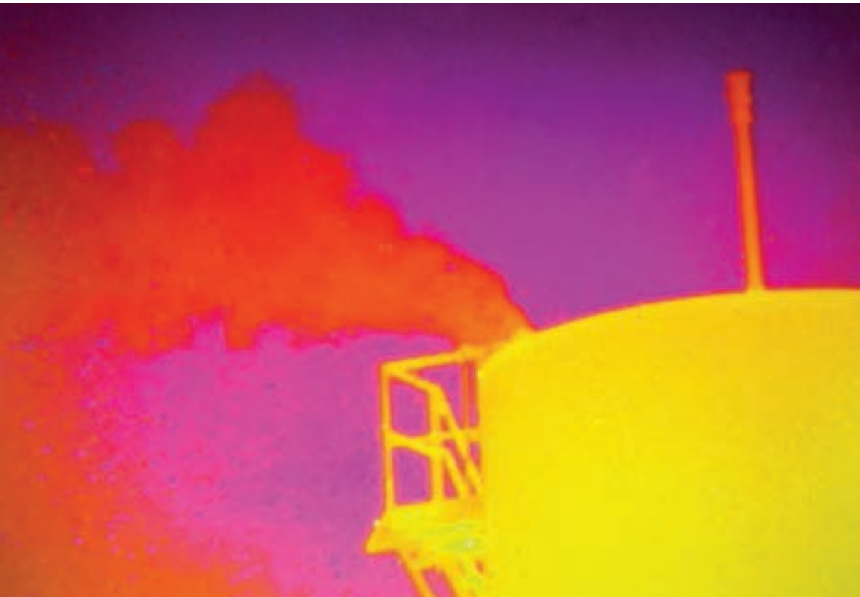
Methane gas escapes from a natural gas storage tank near Aztec, New Mexico, in this thermal camera image captured by Andrew Thorpe of NASA's Jet Propulsion Laboratory. SHAUN STANLEY
