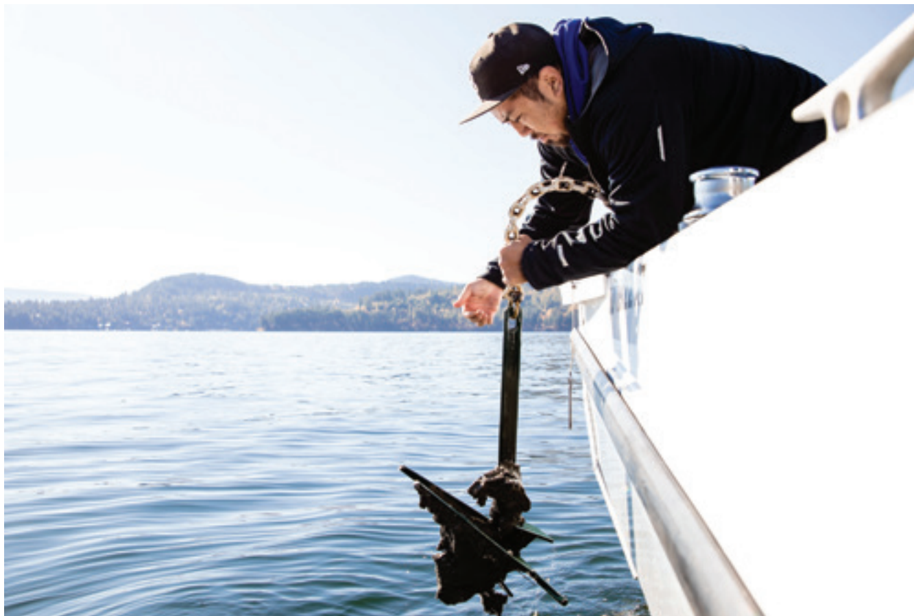
Michael George, a water resources technician for the Coeur d'Alene Tribe's Lake Management Department, retrieves a sediment-covered anchor from the bottom of Coeur d'Alene Lake during a data collection trip in October. The amount of organic materials and nutrients in the sediment are indicators of excessive nutrient loading from the lake's watershed.
