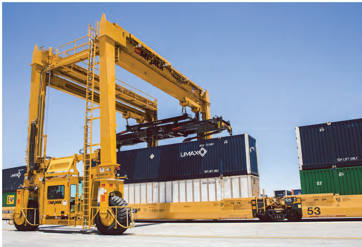
◀ A crane unloads a shipping container from a Union Pacific train at the Santa Teresa Intermodal Ramp.
