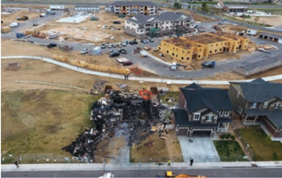
A gas well, seen in the upper left below the bike path, lies less than 200 feet from the Firestone, Colorado, home that exploded in late April, killing two. Investigators say the cause was a “fugitive gas leak” from a well flow line that had been cut but not capped. RJ SANGOSTI/THE DENVER POST VIA GETTY IMAGES
