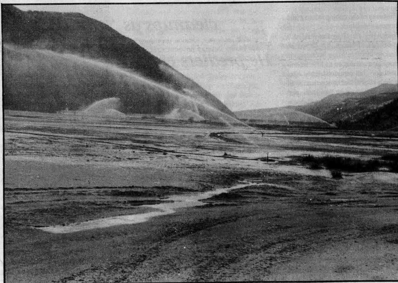
Idarado waters one of its massive tailings mounds
