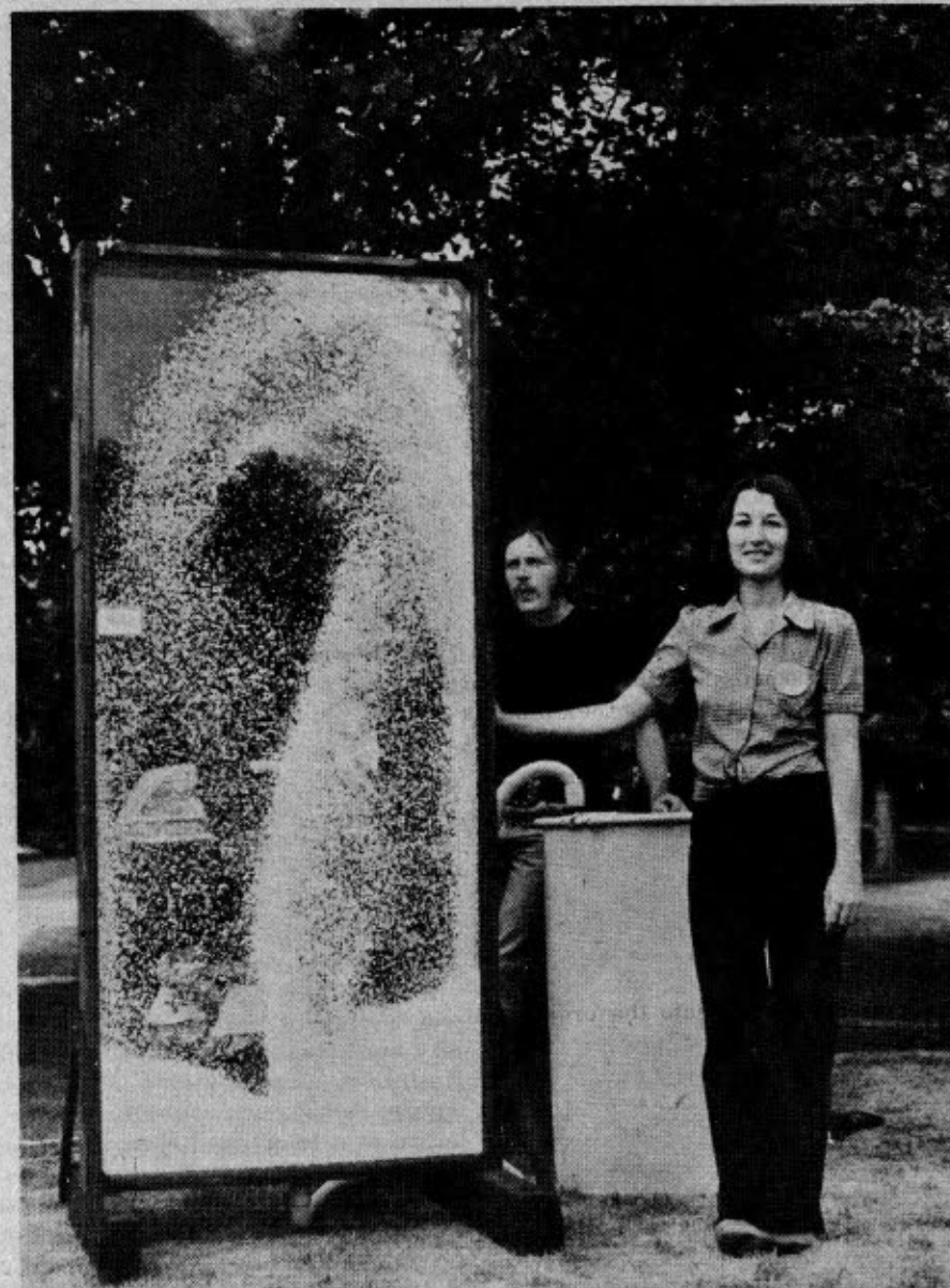
THE AMAZING BEADWALL. A beadwall is an insulated window. To seal up a house, styrofoam beads are blown between the sheets of a double-glazed window with a vacuum cleaner motor. When not in use the beads are stored in a 55-gallon drum. Beadwall plans and a license to build the patented device are available for $15 from Zomeworks, Box 712, Albuquerque, N.M. 87103. The model shown here is a part of the Sunshine Company traveling solar exhibit, sponsored by the University of Denver.
