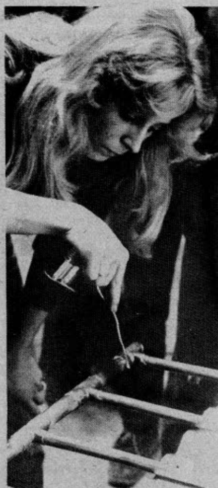
SWEAT SOLDERING THE WATER GRID. Sweat soldering is not difficult, but some instruction is recommended. Here a student from Kelly Walsh High School in Casper, Wyo., is learning how.
