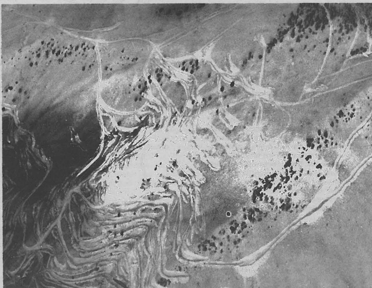
Wyoming's new mining act was strengthened by requiring reclamation of bulldozer exploration for minerals. As the photo above illustrates, exploration can be potentially as damaging to the land and water resources as mining itself. The bulldozer work shown here was done on steep slopes in Wyoming but it is a prevalent practice throughout the West. Federal legislation should also be enacted to protect public lands.
