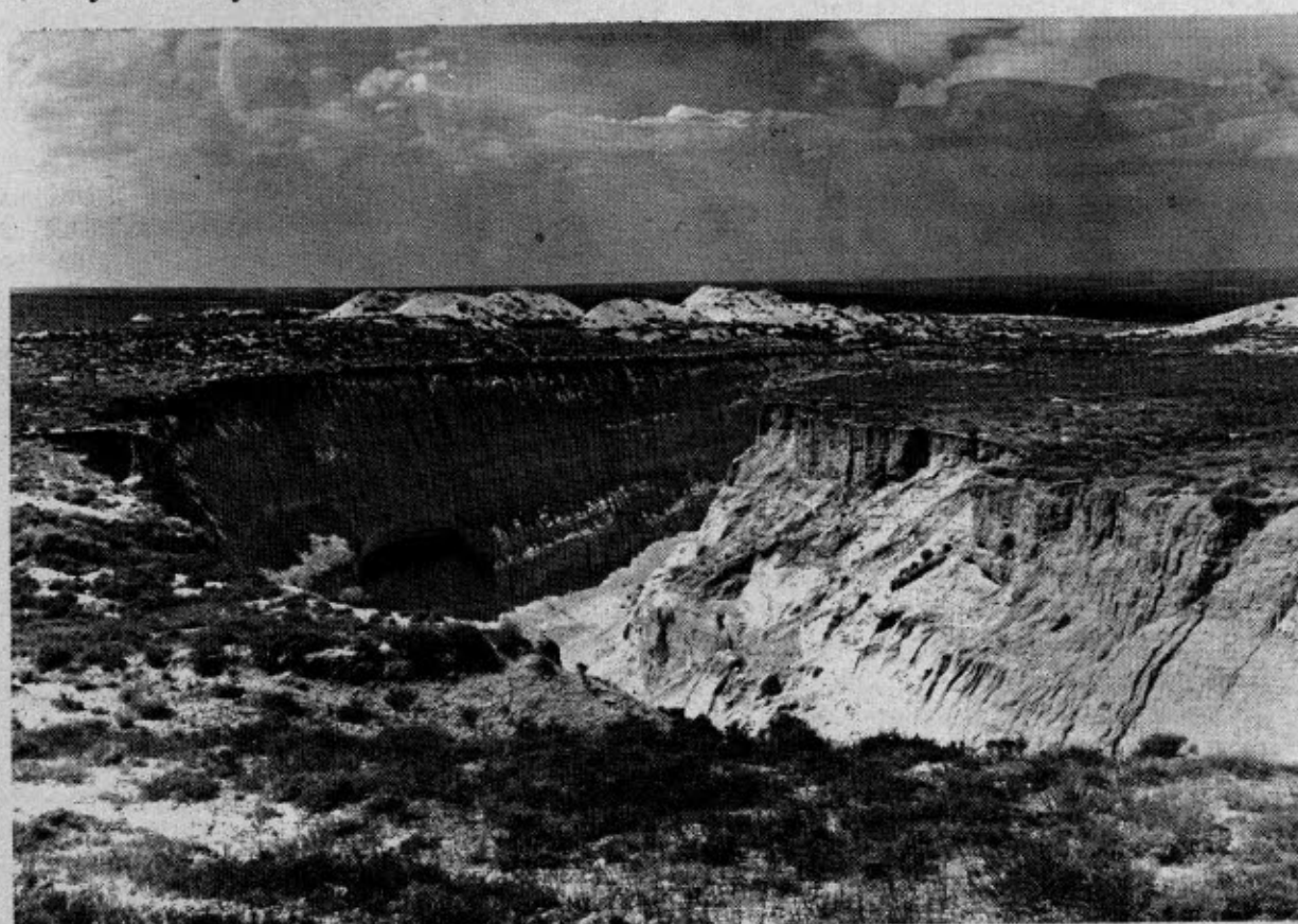
This open pit is all that remains from a uranium mining operation in Wyoming's Gas Hills. The highwalls of the steep, open cut have been left to slough and fall until at some distant, future time natural forces heal the wound. Wyoming's Open Cut Land Reclamation Act makes no provision for the restoration of the highwall. Wyoming's Land Commissioner, A. E. King, who administers the law recently praised the Wyoming Mining Association "for doing a good job of reclamation." He denied charges by environmentalists that the law was inadequate to maintain a quality environment. By its own admission, the mining industry wrote the present law.
