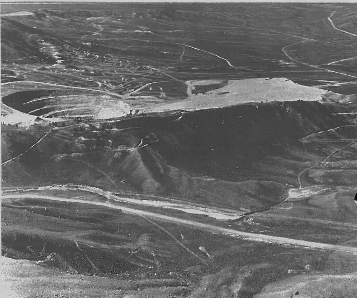
"There is no way to consume power without producing some kind of environmental pollution which must be handled . . ." One of the most serious environmental impacts is that produced by the exploration for and mining of fossil fuels and uranium ores. This steep-sided, deep open-pit has been mined out. It and the ever-present overburden and tailings pile remain for posterity. It is part of the uranium mining area in Wyoming's Crooks Gap in Fremont County.
